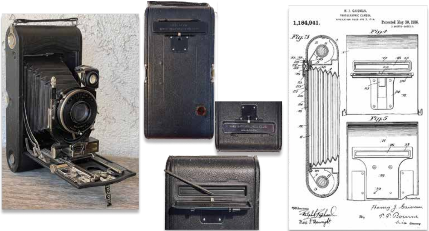
Figure 4: Example of a ca.1915 Kodak Autographic Special 3A with coupled rangefinder that made 6-3 1/4" x 5 1/2" postcard format negatives on No. 122 roll film. Details of the back show the trap door and stylus in bracket, and the open autographic door for access to paper backing of the film and stylus. With a reproduction of the 1916 patent for the autographic feature. [Collection of the author]
