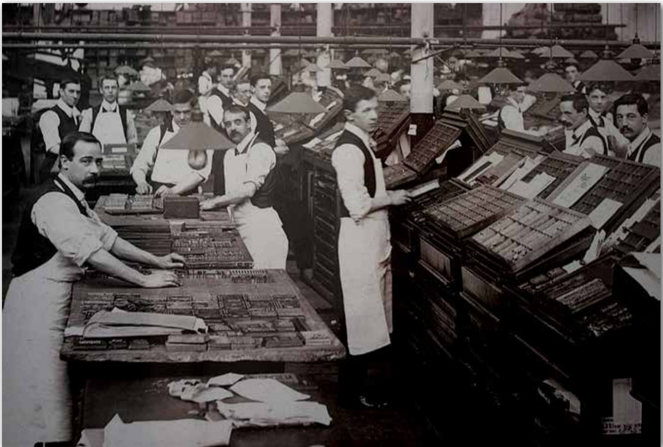
Composition room, 1930s. The men on the left are ‘imposing’ multiple pages by arranging and locking type into chases so that, when eventually printed and folded, the sheets appear in consecutive order. Courtesy of the Printing Collection, Department of Typography, University of Reading.
