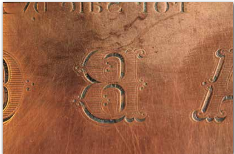
Detail of an engraved copperplate, date unknown. The letterform is Tuscan styled with bifurcated serifs and a drop shadow. The ability to create such extravagant characters, and the capability to stretch or condense them at will, gave the engraver a huge advantage over the letterpress compositor whose letterforms came readymade in fixed sizes. Courtesy of the Printing Collection, Department of Typography, University of Reading.
