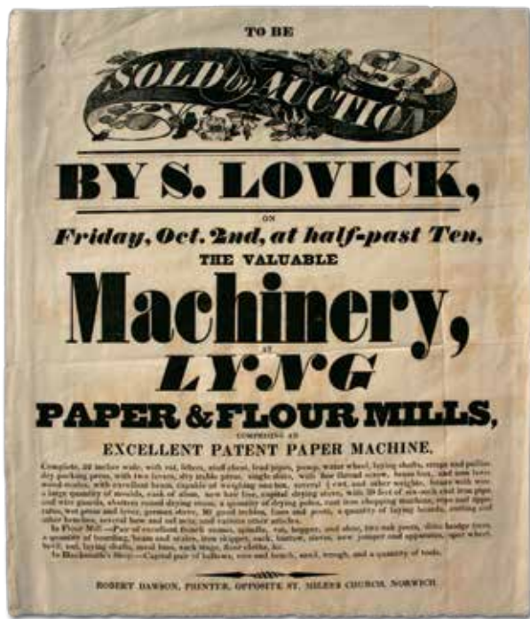
Poster for an auction, letterpress printed by Robert Dawson, Norwich, 1830s. Display typefaces changed the way posters worked and gave the compositor additional responsibilities. In an attempt to provide the poster with maximum impact, the compositor now acted as editor by reducing the size of extraneous copy and increasing the prominence of salient words. Eventually, words such as 'on' and 'at' would be considered extraneous. Courtesy of John Hall.
